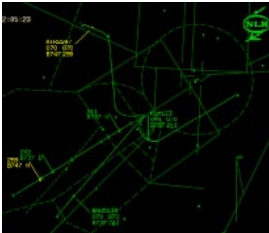
Fig. 14 Picture of the air traffic controller "ghosting" display aid for CDA approach
