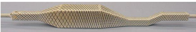
Figure 3. The preform of a complex-shaped hollow component as an example of a biaxial braid
