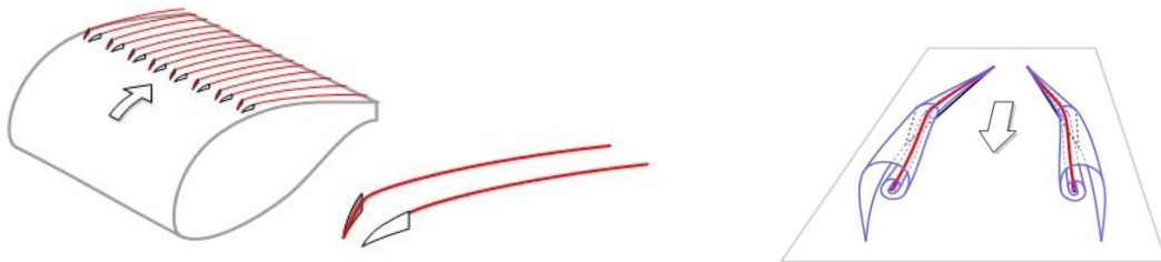
Figure 4 Thick trailing edge airfoils and vortex generators for wind turbine applications.
