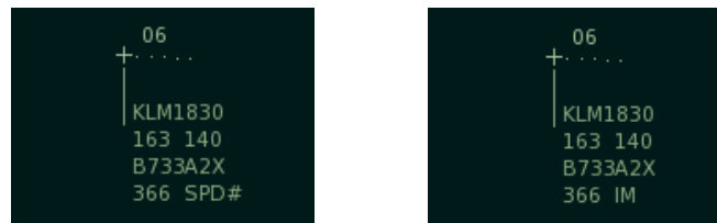
Figure 4. Track labels showing aircraft eligible for IM Operations (#, left) and aircraft engaged in IM Operation (IM, right).
