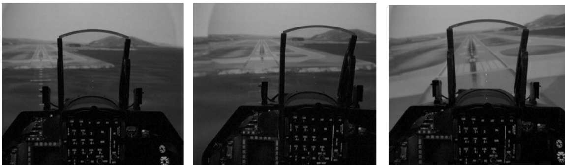
Fig. 3 Time-lapse images from inside the cockpit showing the sequence of the simulated decrab maneuver (from left to right).
