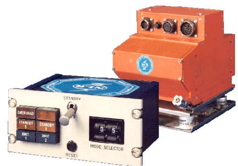
Figure 1 NLR Smart box unit and panel
