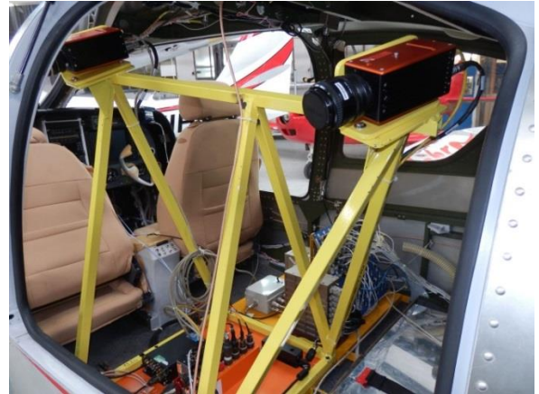
Figure 5 EVEKTOR Cobra with a speckled pattern taped on the left wing and cameras installed in the cockpit
