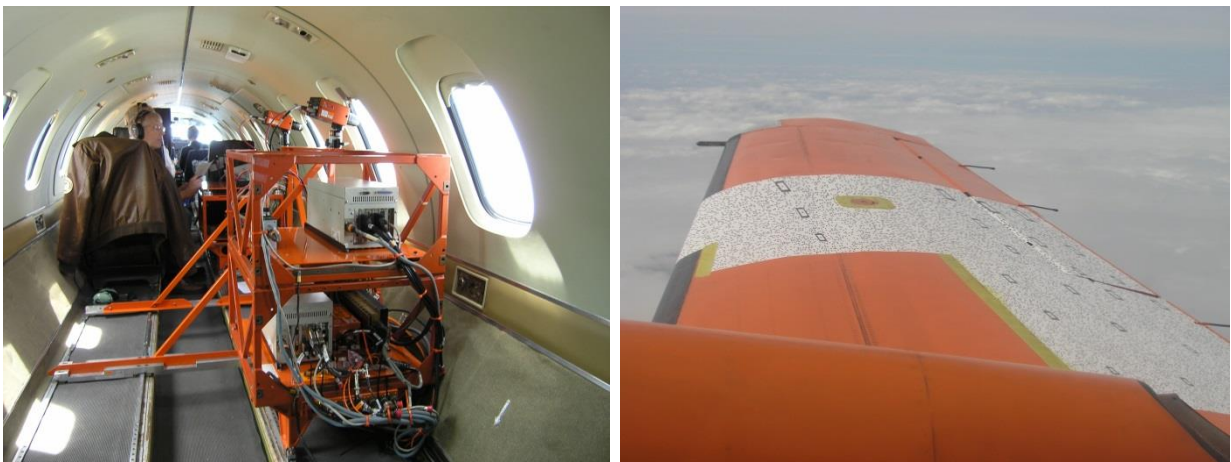
Figure 4 Pictures of the interior of the NLR Fairchild Metro during the AIM 2 flight test (left) and of the starboard wing of the aircraft with the partly speckled wing, aileron and flap (right picture)
