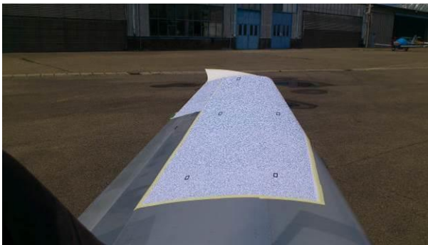
Figure 5 EVEKTOR Cobra with a speckled pattern taped on the left wing and cameras installed in the cockpit
