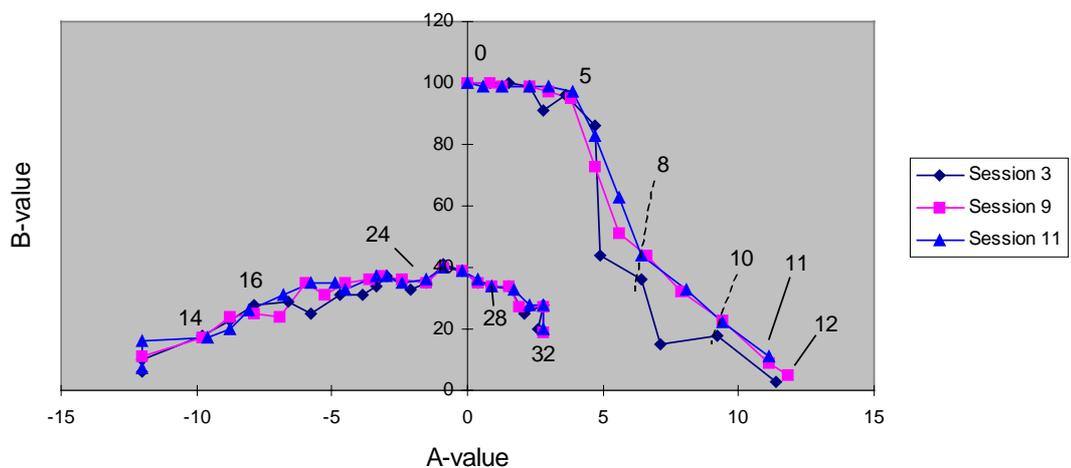
**Fig. 8 Fokker Bondtester A/B values for the flat-bottomed holes in the Glare 4B-32/31-0.4 panel. Three independent measurements with crystal 5410 (diameter 1.25 inch). The numerals indicate the depth in aluminium layers**
