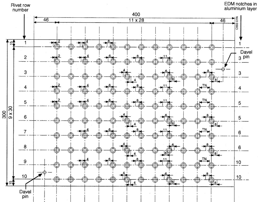
Fig. 3 Schematic diagram of the Glare 4B-5/4-0.4 lap joint specimen with EDM notches
