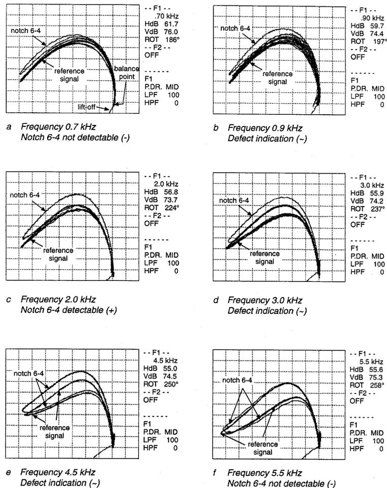
**Fig. 6 Determination of the optimum eddy current test frequency (about 2 kHz) for the sliding probe inspection of notch 6-4 (length 4 mm, at a depth of 6 Al layers) in the Glare 4B-0.4 lap joint specimen**
