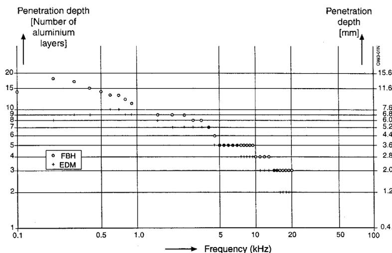
**Fig. 5 Eddy current penetration depth in Glare 4B-0.4 laminate as function of the test frequency. Optimum performance of the surface probes**
