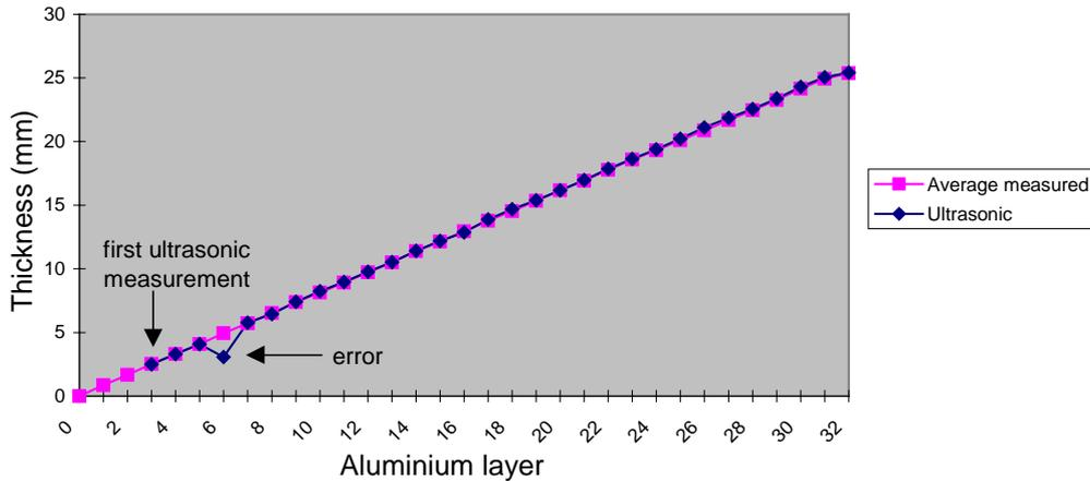
**Fig. 10 Ultrasonic depth measurements for the flat-bottomed holes in the Glare 4B-32/31-0.4 panel. Comparison with actual values (average measured)**
