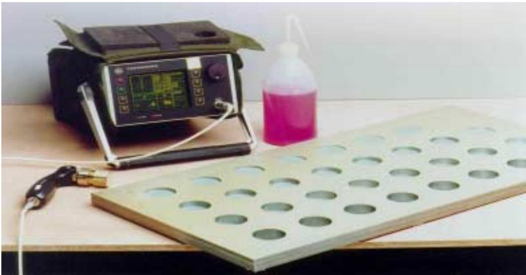
**Fig.2 The Fokker Bondtester Model 90 and the Glare 4B-32/31-0.4 test panel with flat-bottomed holes**
