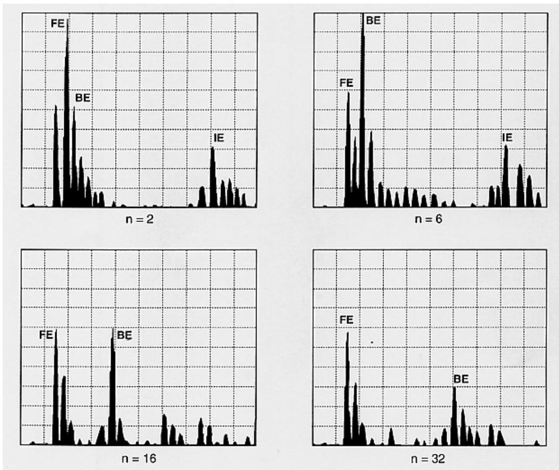
**Fig. 9** Ultrasonic pulse-echo responses for a Glare 4B-0.4 test panel with  $n$  layers (FE: front echo of the test panel, BE: back echo of the test panel, IE: internal echo in the transducer/delay line)
