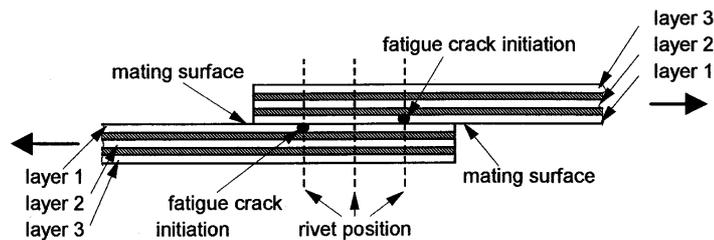
Fig. 4 Cross-section of a Glare 3/2 riveted lap joint with the first crack initiation locations (Fig. 4.6 from Ref. 2)
