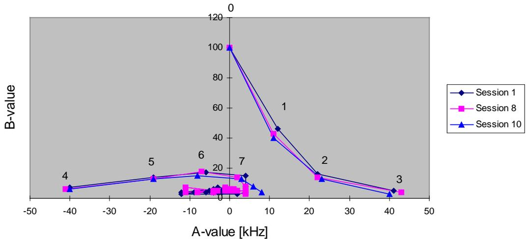
**Fig. 7 Fokker Bondtester A/B values for the flat-bottomed holes in the Glare 4B-32/31-0.4 panel. Three independent measurements with crystal 1414 (diameter 0.25 inch). The numerals indicate the depth in aluminium layers**
