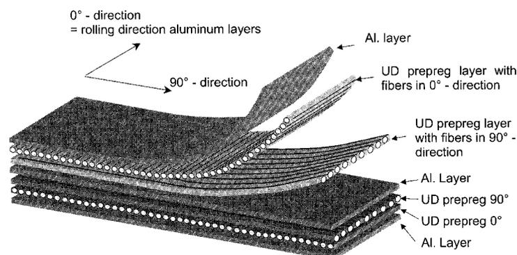
**Fig. 1 Schematic of a Glare laminate with 3/2 lay-up: three aluminium layers and two intermediate prepreg layers with glass fibres in the 0°- and 90° direction**
