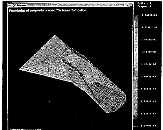
Fig. 7b Thickness distribution after optimization
