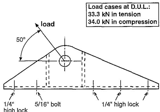
Fig. 2 Static load cases for the metal bracket
