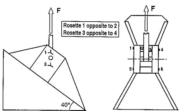
Fig. 12 Test set-up and instrumentation of the bracket
