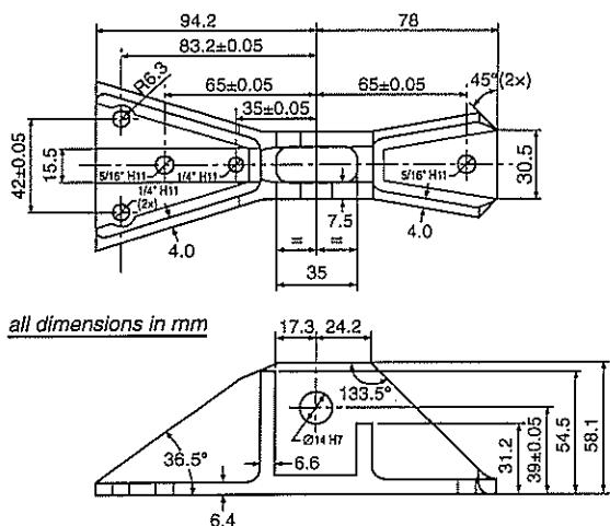
Fig. 8 Dimensions of the composite bracket after optimization
