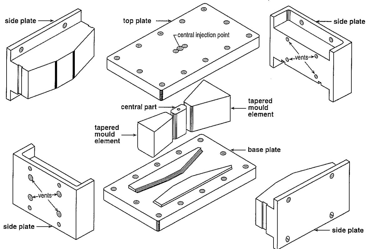
Fig. 10 Elements of the RTM mould
