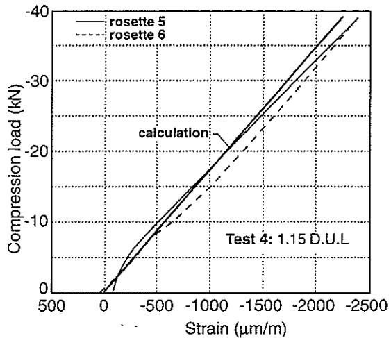
Fig. 13 Calculated and measured load-strain curves
