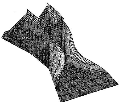
Fig. 9 First buckling mode at 8.5 Design Ultimate Load
