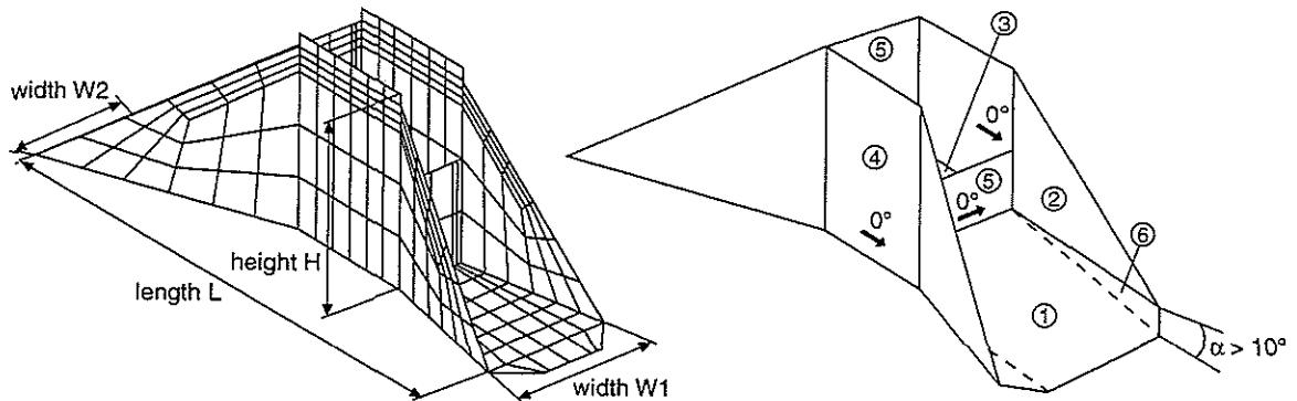
Fig. 4 Geometric design variables and sections 1 to 6
