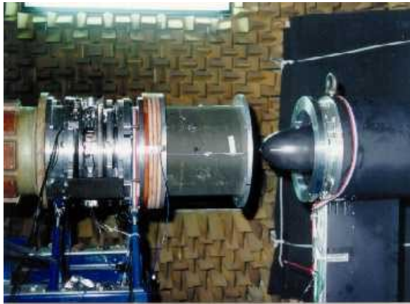
Fig. 3 Liner barrel connected to fan model in NLR's anechoic wind tunnel KAT
