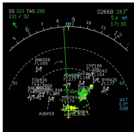
Figure 4: Navigation display with bigger aircraft symbols, with traffic and weather located closer to the own ship. BIGGER & CLOSER
