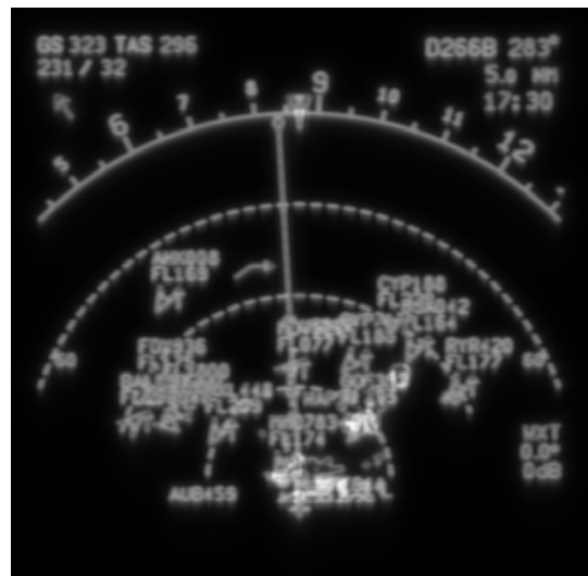
Figure 8: Full clutter map of display with bigger symbols, and with traffic and weather located closer to the own ship. BIGGER & CLOSER: Clutter = 12.13
