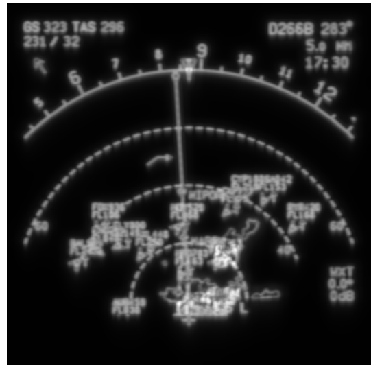
Figure 7: Full clutter map of the display for which traffic and weather are located closer to the own ship. CLOSER: Clutter = 11.42
