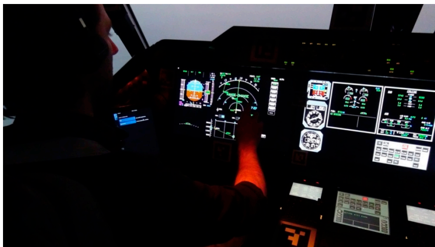
Fig. 2. Picture of the touch input display including the late runway change tool
