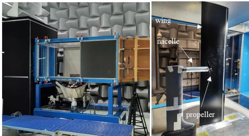
**Figure 3 a) Exterior of the test section in the AWT, b) F15 wing model and nacelle with the propeller in the test section b). Note that one wall has been removed when taking these images.**
