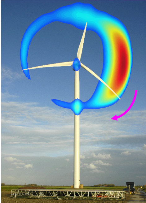
Figure 20 A typical modern large wind turbine. The noise source distribution in the rotor plane (averaged over many revolutions) is projected on the picture
