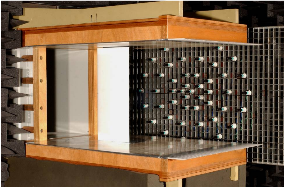
Figure 11 NLR's small anechoic wind tunnel KAT with white airfoil model between endplates and out-of-flow microphone array
