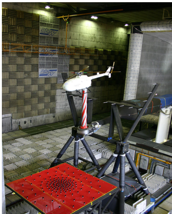
Figure 52 Helicopter model in DNW-LLF wind tunnel, with (red) out-of-flow microphone array
