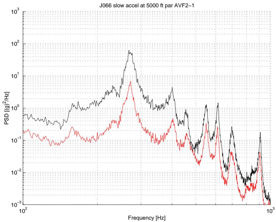
Figure 3. Power Spectral Density plot of right forward ventral fin accelerometer, red: without tgt pod, black: with tgt pod.
