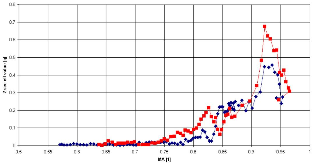
Figure 2. LCO (effective g) level measured at left hand wing tip launcher, with pods (blue) and without pods (red).
