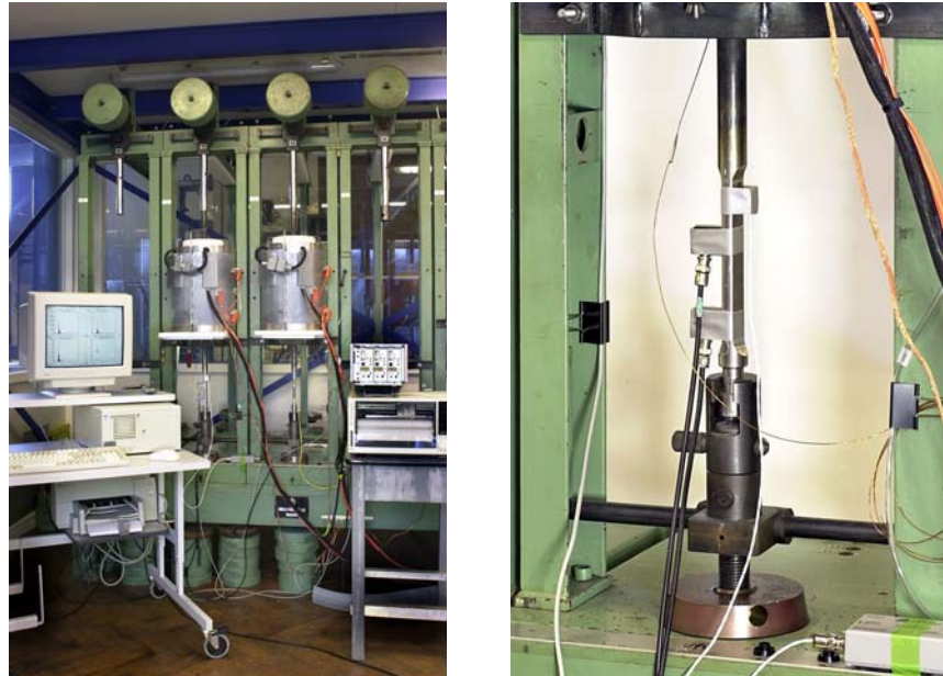
Fig. 6 Test set-up with the creep bank (with split furnace), AE equipment and the position of the AE sensors
