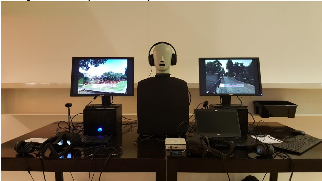
Fig. 4 – The set-up for Lelystad Community meeting with two VCNS systems and in the middle the dummy head for calibration purposes.
