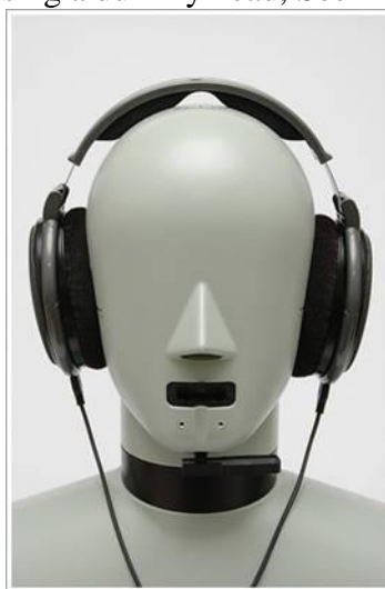
Fig. 1 – A dummy head with microphones in the ears is used for the calibration of the simulator.
