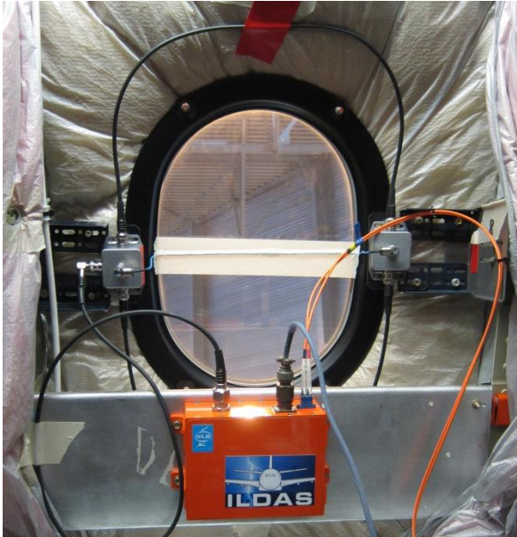
Figure 6 – Installation of the magnetic-field window sensor
