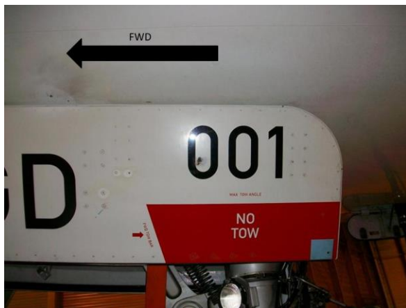
Figure 17 – The left nose landing gear door with minor damage in the '001' lettering
