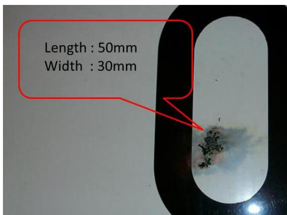
Figure 18 – Detailed view of nose landing gear damage
