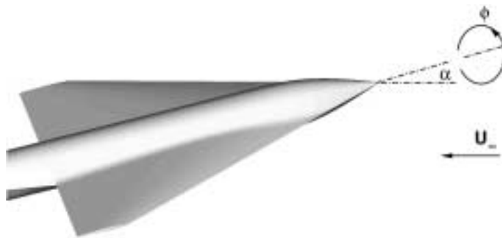
Fig. 2 Roll-motion about the body axis.
