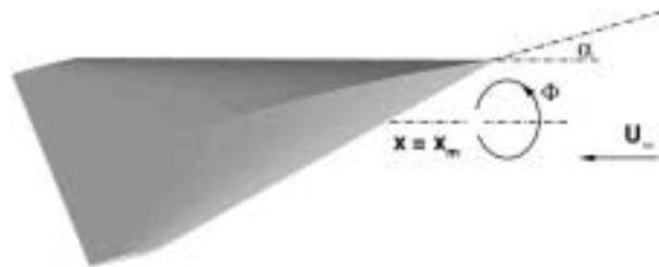
Fig. 3 Roll-motion about the wind axis.
