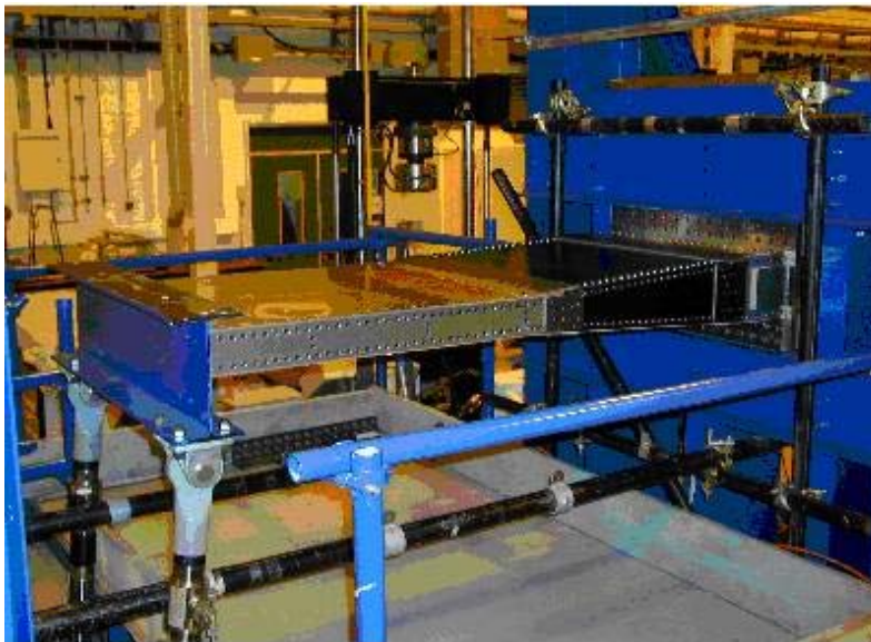
Fig. 2 Modular wingbox under test at QinetiQ
