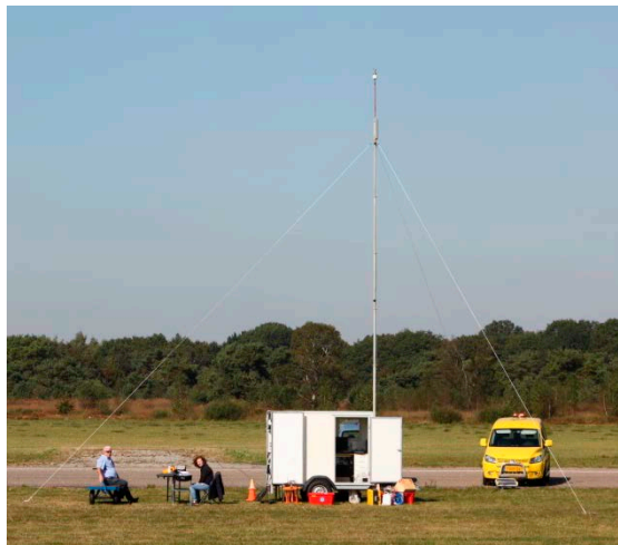
Figure 7: Ground station with weather measurement mast.
