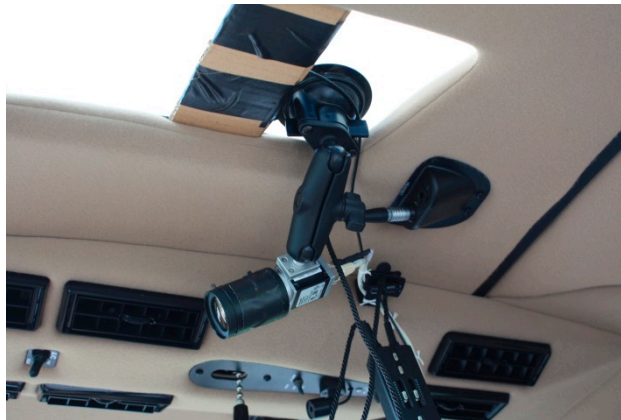
Figure 3: Smartcam as installed on R66.
