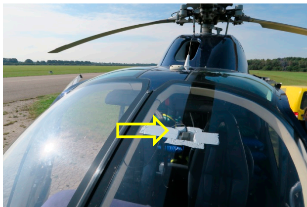
Figure 1: GNSS antenna as installed on EC120.
