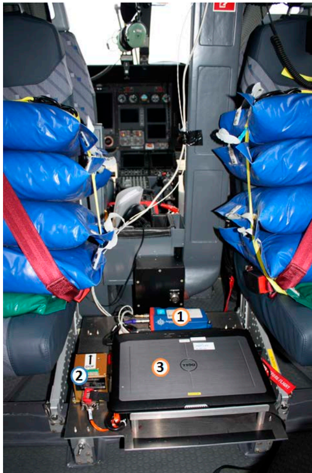
Figure 5: COFDR as installed in the EC135 to the seat rails of a removed seat with 1) GNSS Receiver, 2) IMU and 3) laptop computer.
