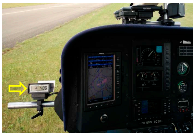
Figure 2: Optical tachometer as installed on EC120.
