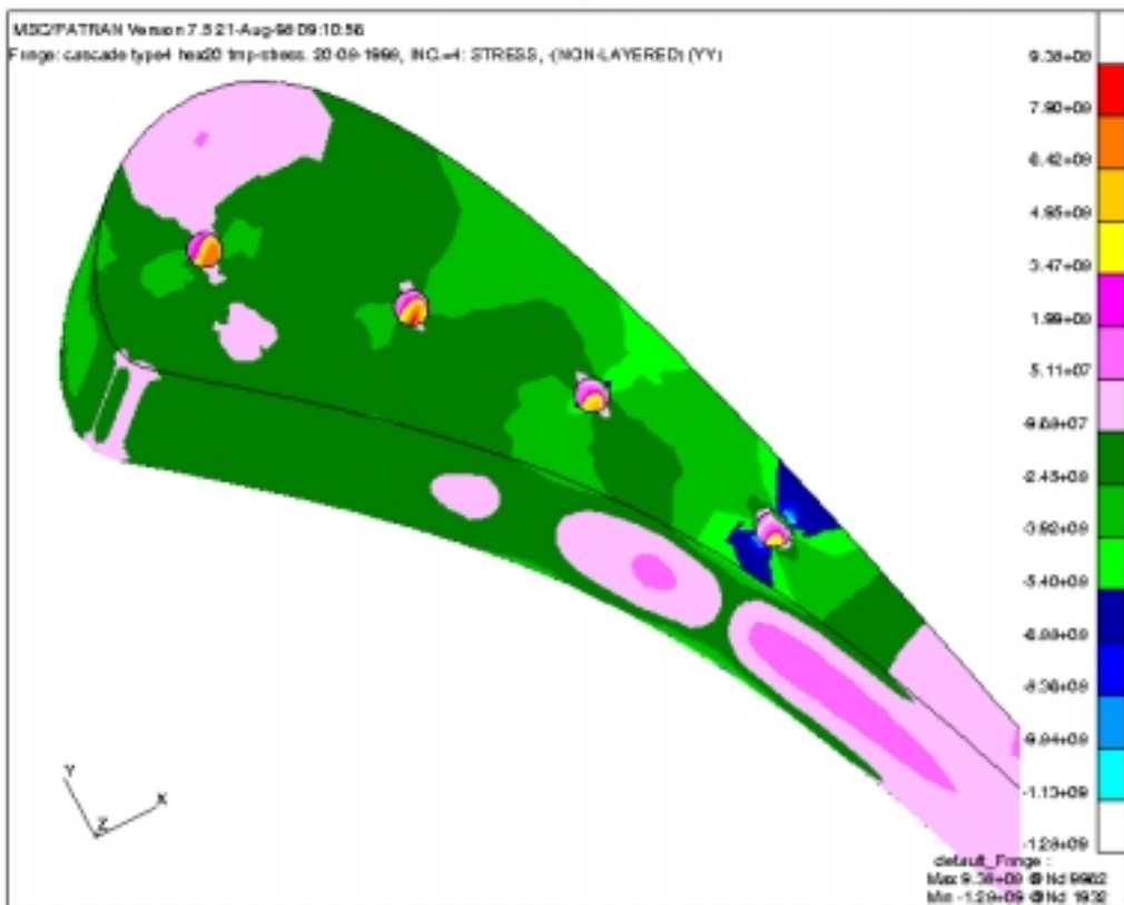
Figure 5 Thermal stresses calculated for an internally cooled blade
