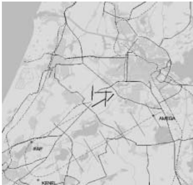
Figure 3: An illustration of the CDA from Northeast on RWY06. This figure shows Schiphol airport, the nominal route (dashed line), the six cross-sections perpendicular to the nominal route. The stars indicate the AMEGA and KENEL waypoints, and the final approach point (FAP).
