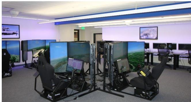
Figure 2 ZedaSoft Zuse Simulation Stations at the USAFA MDL
