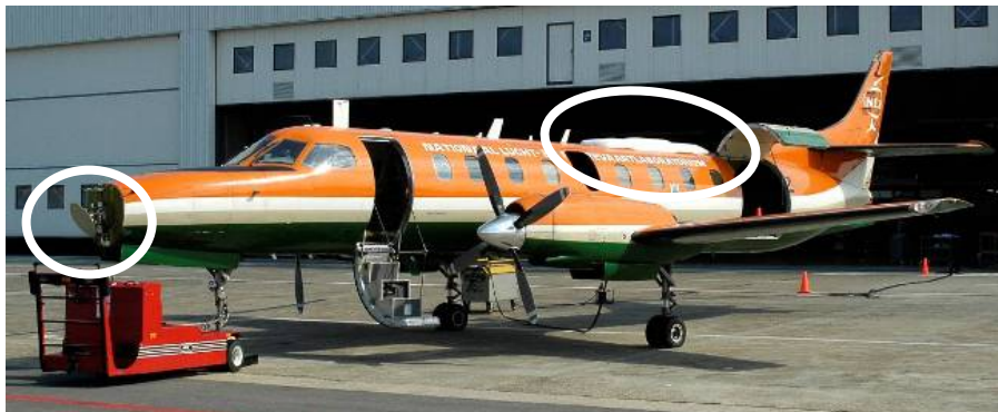
Figure 4 NLR's Swearingen Metro II research aircraft with multiscan weather radar attached on the nose and satellite antenna on top of aft fuselage during preparation for FLYSAFE flight tests in the summer of 2008. See Figure 6 and Figure 7 for details.
