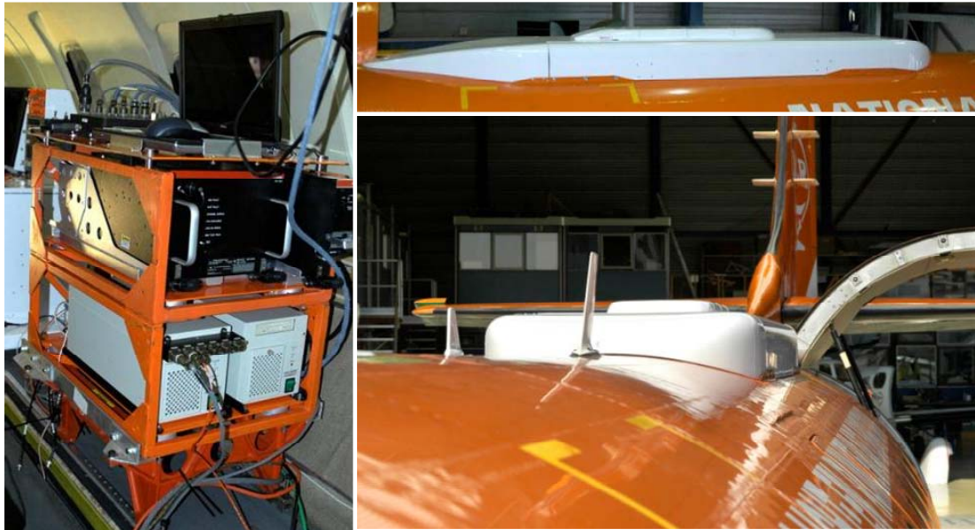
Figure 6 High speed SATCOM system (black coloured boxes in avionics rack on left with SANTA lap-top on top). Side and front view of SATCOM antenna attached to antenna box are shown at the upper respectively lower right.
