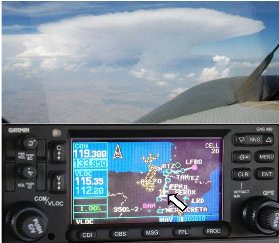
Figure 9 Stormscope detected lightning activity indicated on Garmin 430 (bottom) together with corresponding cockpit view in direction of flight (top). Aircraft symbol is indicated by arrow. Yellow markings at 10-11 o'clock position indicate lightning activity. Test flight over North of Spain via Biarritz to Toulouse.
