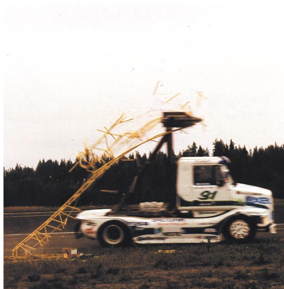
b) Full scale impact at 140 km/h
