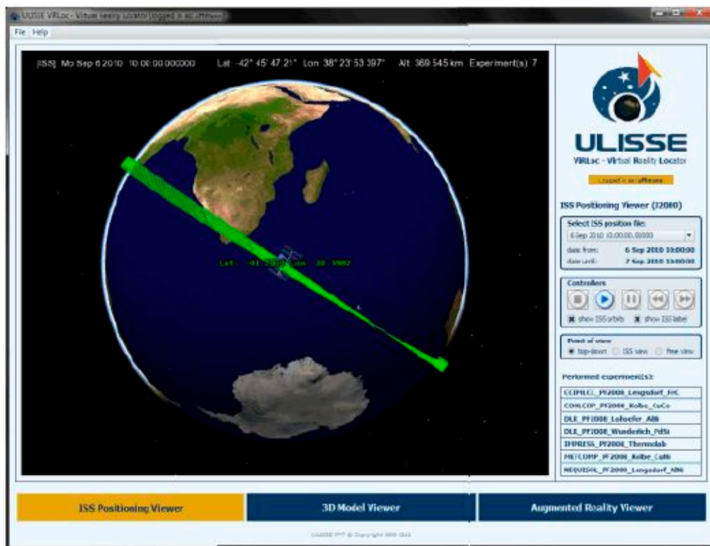
Fig. 7-1. The ISS Positioning viewer of ViRLoc after loading ISS positions with the top-down camera view.
