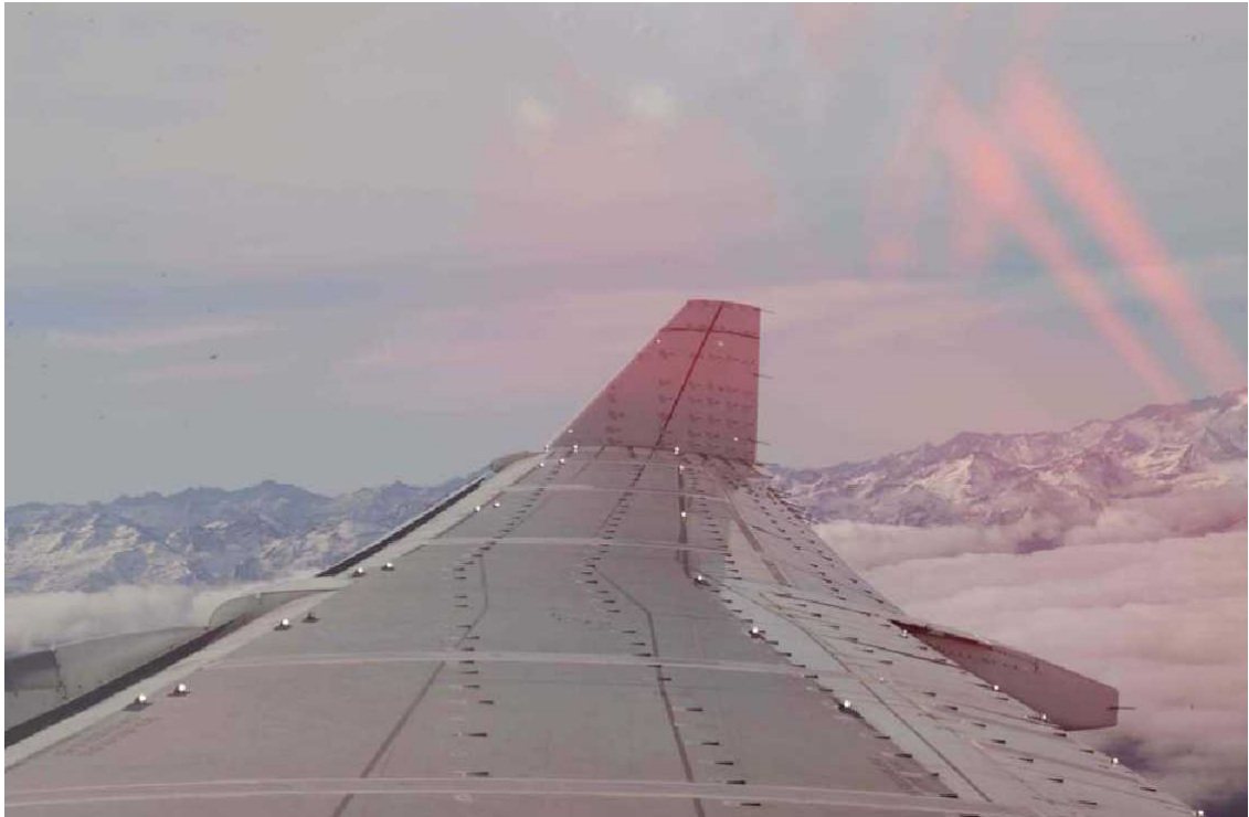
Figure 1 Overview of the targets on the starboard wing for deformation measurement
