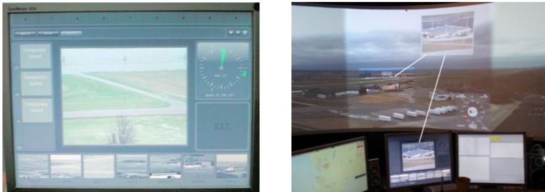
Fig. 2-6 Pan Tilt Zoom camera Human Machine Interface (left) and Picture in Picture (right)
