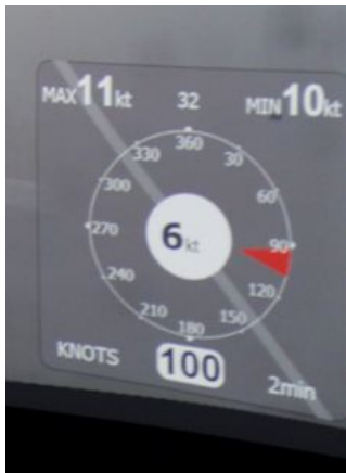
Fig. 2-4 Meteorological overlay with actual wind speed, direction , 2-minute average and minimum – maximum values
