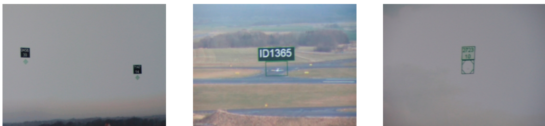
Fig. 2-5 Left: Aircraft tracked only by the Terminal Approach Radar (labels with call sign or SSR code and altitude in hundreds of feet); Middle: aircraft tracked by the video camera only (label with track number); Right: aircraft tracked by both radar and video
