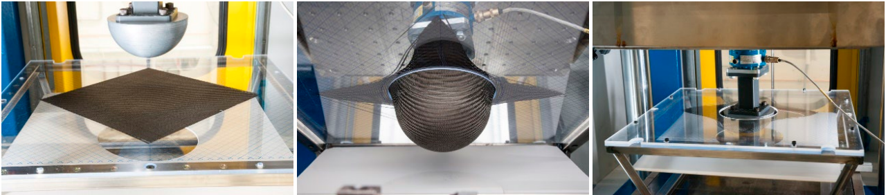
Figure 4: Draping of dry carbon fibre fabric into the double curved sphere shape. This is a common test shape to investigate the shear of the individual yarns of the fabric. At NLR the test was performed with the fabric between two transparent plastic sheets with a central hole and a 3D printed sphere mould was lowered through the transparent plates
