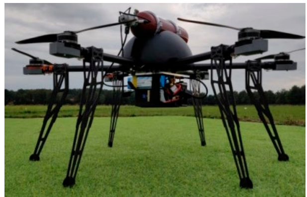
Figure 1 NLR's Hydrogen Drone HYDRA-1A, Size: Ø120 x 60 cm
