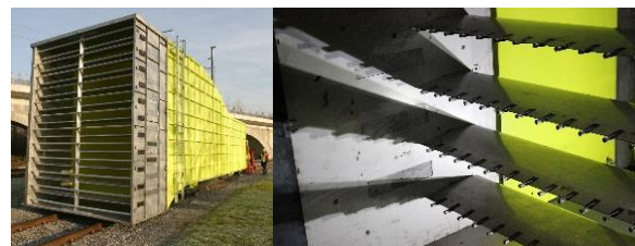
Figure 6: Spray bar system with atomizing nozzles.
