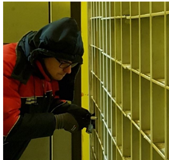
Figure 11: Grid measurement for uniformity check of the cloud condition.
