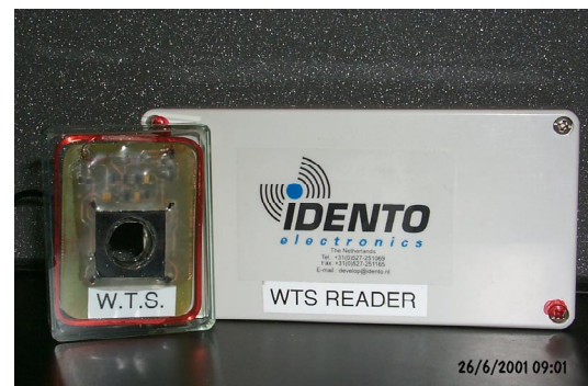
Figure 14. Prototype wireless turbidity sensor using RF field for power and data transfer and remote operation electronics as developed in co-operation with IDENTO Electronics.
