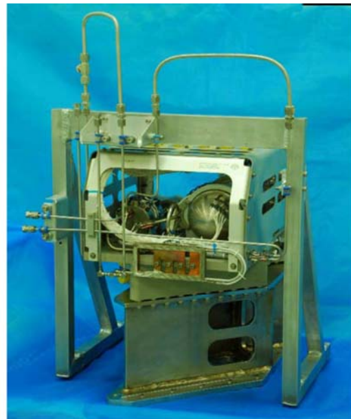
Figure 10: TTCB-P box assembly on USS simulator and in vibration frame (picture by AIDC)
