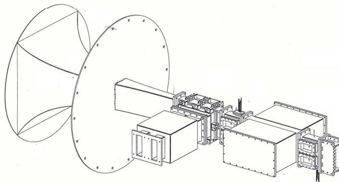
*Figure 1 Hot stream liner test set-up with collector/ contraction, source section, measurement section for the incident acoustic field, liner test section with two boxes, measurement section for the transmitted acoustic field and lined exit nozzle.*
