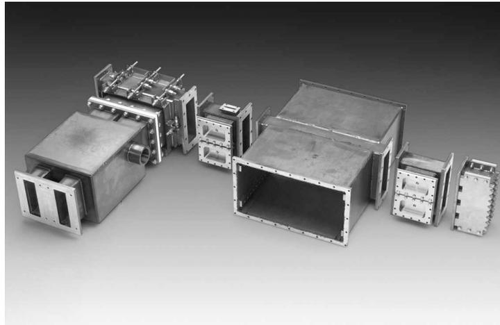
*Figure 2 Duct elements of the NLR hot stream liner test facility.*
