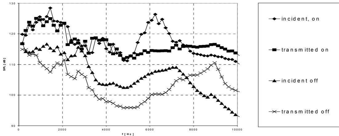
Figure 7 Acoustic signal to flow noise ratio, hard-wall,  $T = 500\text{ }^{\circ}\text{C}$ ,  $M = 0.35$ , loudspeakers are switched on or off (flow noise only), broadband excitation,  $\Delta f = 160\text{ Hz}$ .
