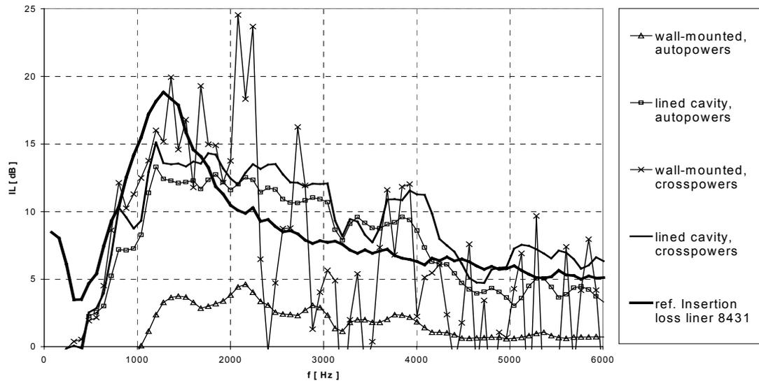
Figure 3 Comparisons of various measured insertion losses in the NLR-FDF, reference liner 8431, flow Mach number is 0.35, broadband excitation,  $\Delta f = 80$  Hz.
