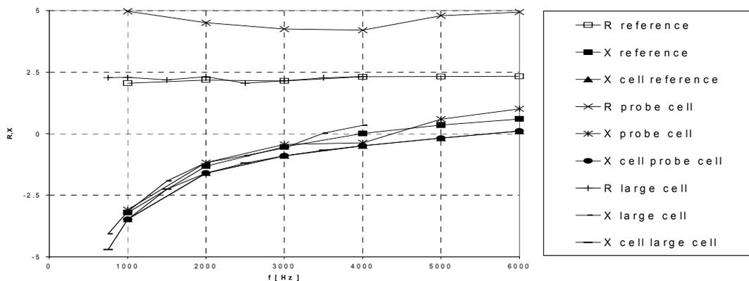
Figure 5 Comparison between measured in-situ acoustic impedances with various techniques,  $Z=R+iX$  ( $X=X_{facing\ sheet}+X_{cell}$ ),  $M = 0.3$ ,  $SPL = 120$  dB, tonal excitation.
