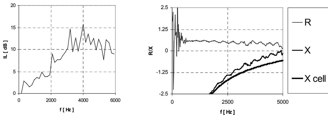
Figure 8a+b Insertion loss (left) and in-situ acoustic impedance,  $T = 440\text{ }^{\circ}\text{C}$ ,  $M = 0.3$ , broadband excitation,  $\Delta f = 160\text{ Hz}$  (a) and  $\Delta f = 20\text{ Hz}$  (b).
