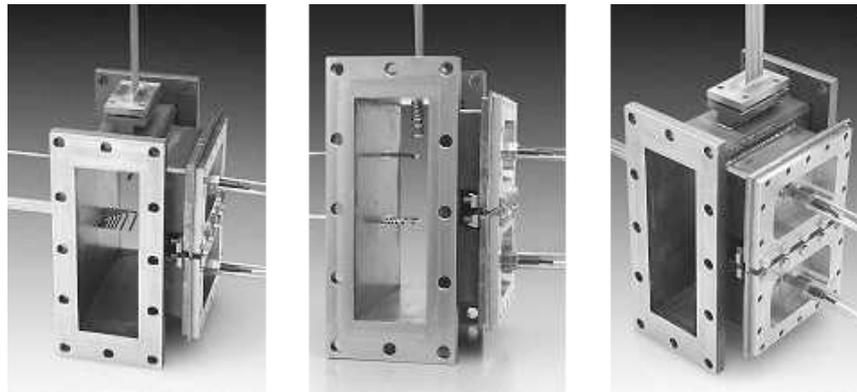
*Figure 6 Measurement sections with acoustic (Kulites at right side) and aerodynamic instrumentation for transmission and insertion loss measurements.*
