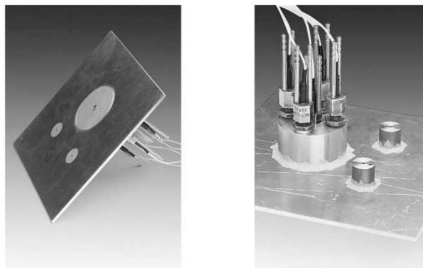
Figure 4 Test sample to validate various in-situ acoustic impedance measurement techniques (reference cell, probe cell and large annular cell).
