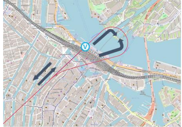
Figure 1. Departure and arrival routes (red) for the hypothetical Vertiport located at Amsterdam Central Station (arrows depict the flight directions).
