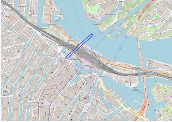
Figure 3. IR contour 10^{-6} /year (blue) for 700 eVTOL movements a year.
