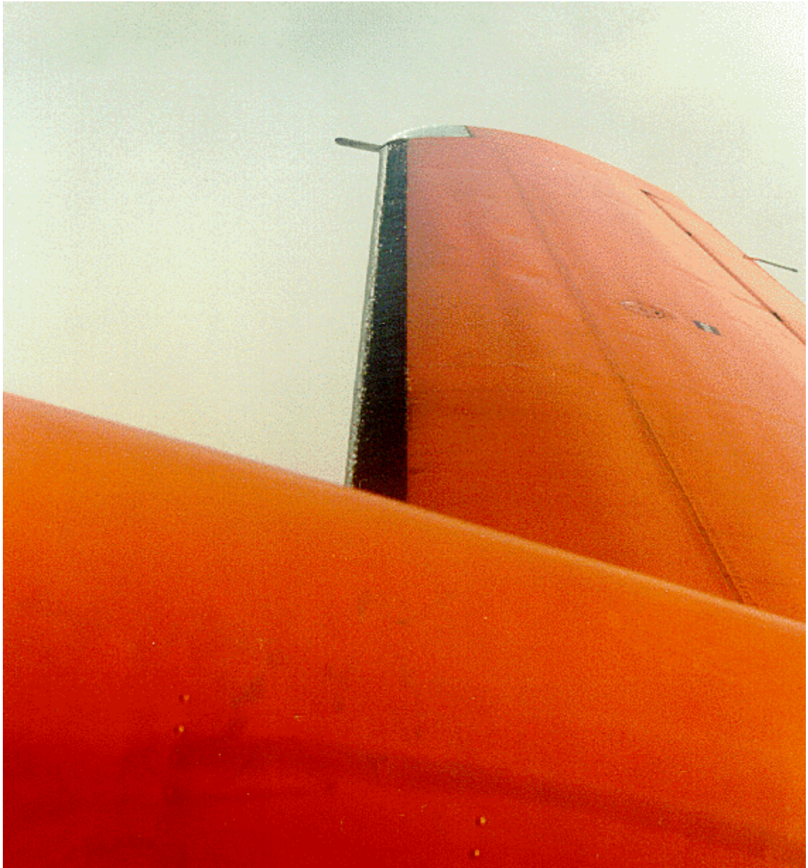
Fig. 7 Photograph of ice accretion on the wing of the research aircraft. Ice accretion is close to the leading edge of the wing on the de-icing boot.
