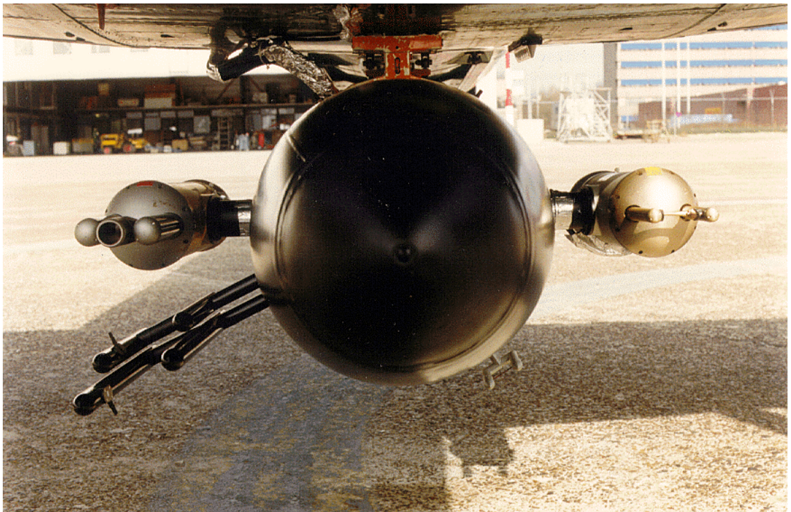
Fig. 3 The pod with cloud physics instrumentation installed under the NLR research aircraft
