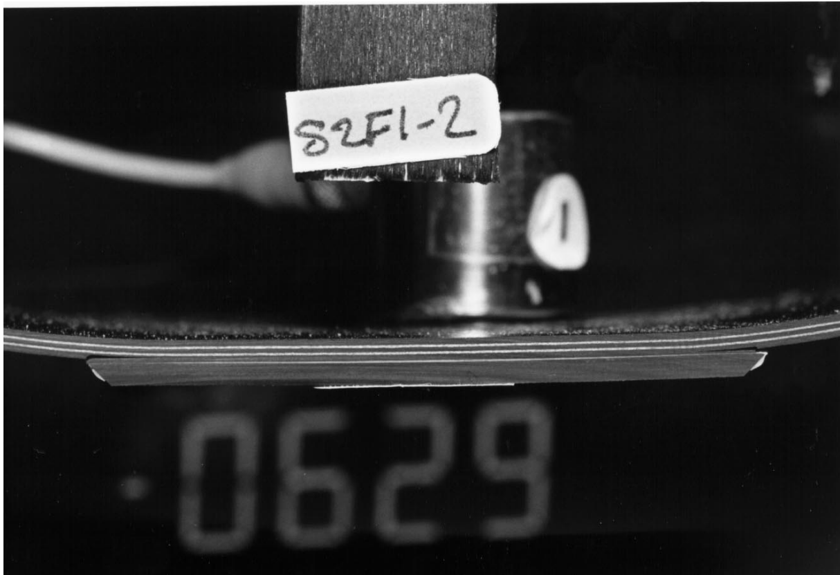
Figure 4 Photograph of specimen S2F1-2 containing delaminations on either side.
