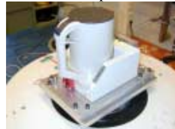
Figure 2 The shaker testing a water boiler
