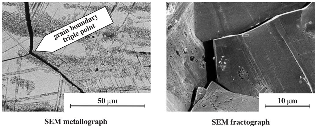
Fig. 3 Microstructurally-induced brittle intergranular fracture (Wanhill *et al.* 1998)
