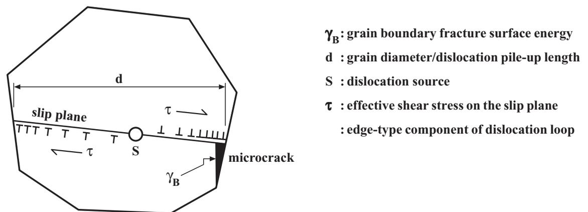
Fig. 7 Nucleation of a microcrack by dislocation pile-up. Under the shear stress  $\tau$  the source  $S$  generates dislocation loops which pile-up at barriers (the grain boundaries) in the slip plane. The resulting stress concentrations nucleate microcracks at one or both of the barriers. After Lawn (1993, 318) and Thompson and Knott (1993)
