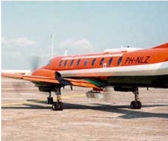
Fig. 2 The Fairchild Metro II research aircraft. This aircraft has the exhaust in sight of cabin windows, enabling easy installation of open-path spectrometers.
