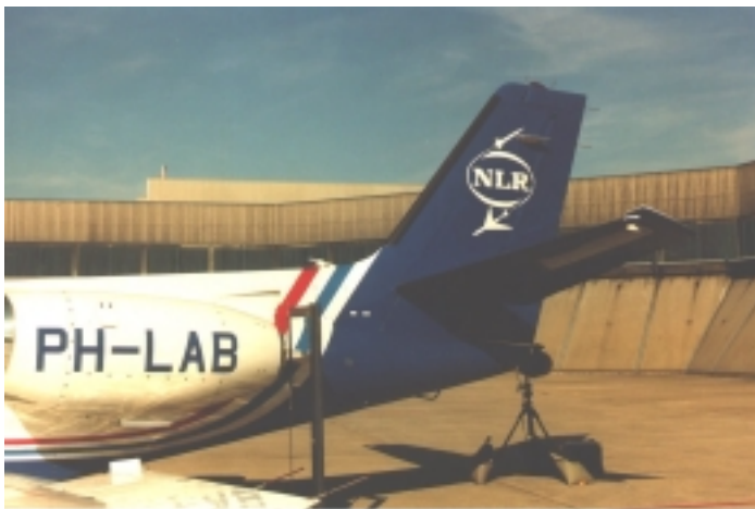
Fig. 1 Set-up for evaluating spectrometers. Gas samples are taken from the perforated tube installed behind the exhaust of the engine and led to gas analysers. A retroreflector is visible behind the tail of the aircraft
