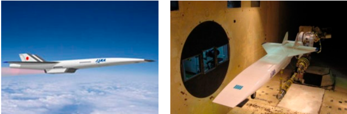
Figure 1: Hypersonic passenger aircraft concept, left: artist impression of JAXA HST, right: Low-speed wind tunnel test ( http://www.aero.jaxa.jp/eng/ ).
