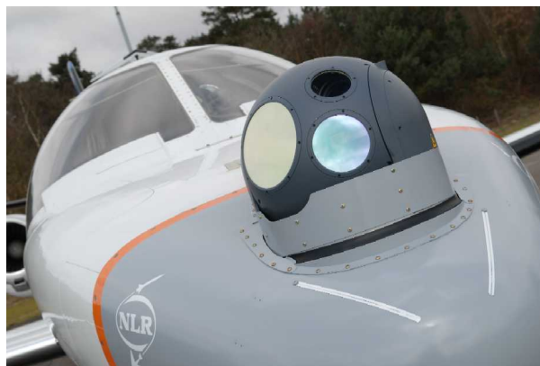
Fig. 1 Final and certified situation of camera installed on Cessna Citation 2
