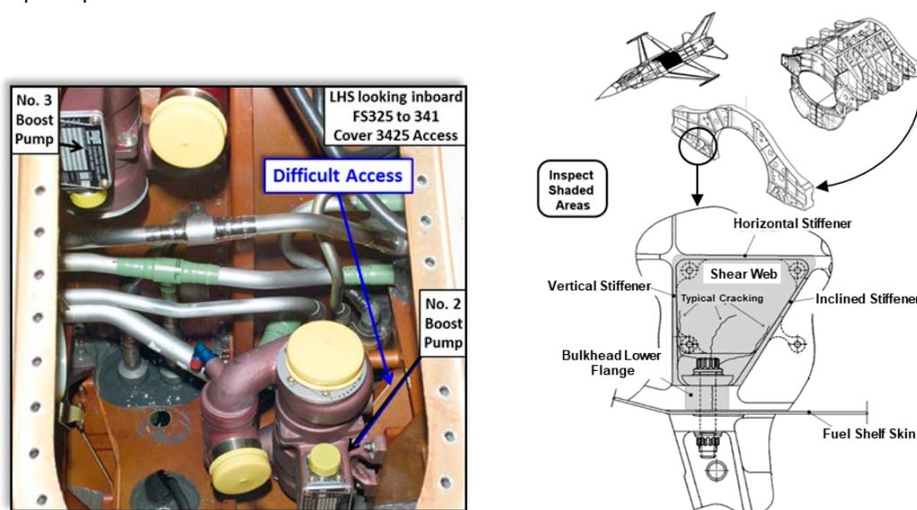
Figure 4: Difficult access to the fracture critical F-16 fuel shelf joint bolt holes (left), easy visual inspection for large cracks in flanges and web of the upper bulkhead (right) (Jones et al., 2012).
