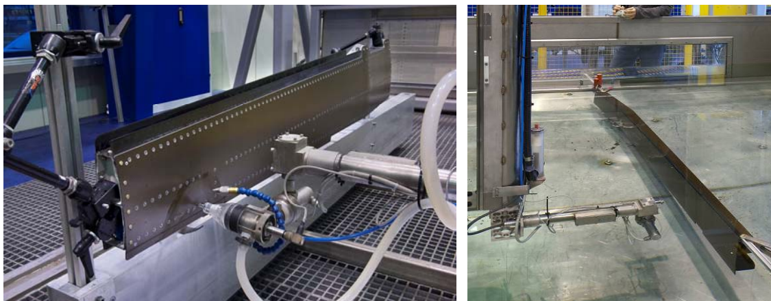
Figure 13. Squirter and immersion inspection at NLR of wingbox respectively co-bonded lower skin
