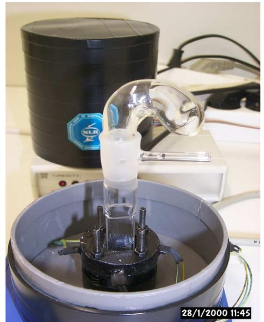
Figure-4. Optical sensor head breadboard with cuvette
