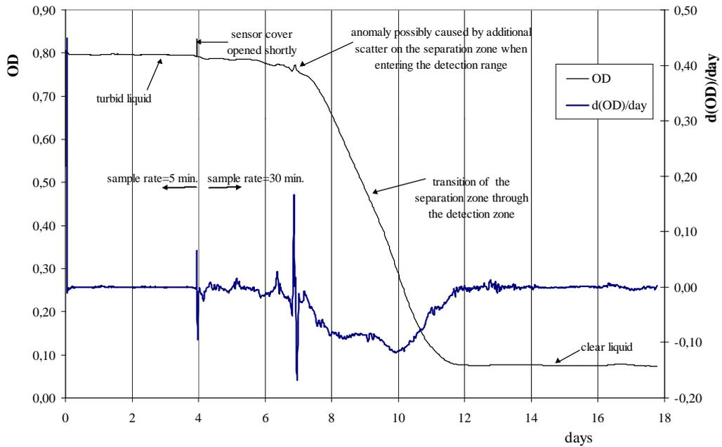
Figure-6. Presentation of the OD value obtained from the real-time measured sensor signal (OD calibrated versus  $\ln R^*$ ) when the separation zone passes the detection zone of the sensor, with the calculated OD rate (OD/day) included.
