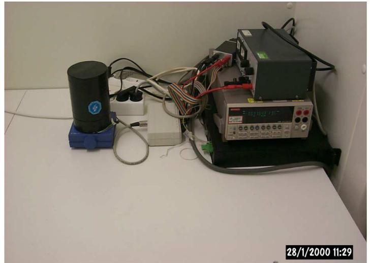
Figure-9. The biomass sensor breadboard set-up on a table in the temperature-controlled room at BIOCLEAR. Note the magnetic stirring device on which the sensor head is placed.
