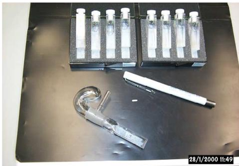
Figure-7. Overview of the measurement cuvettes. One measurement cuvette with air reservoir. Eight measurement cuvettes, filled with liquid medium and fixated bacteria of various concentrations for calibration purposes.
