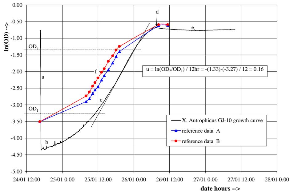
Figure-10. *X. Autrophiacus GJ-10* growth curve, with geometrical estimation of the maximum growth rate ( $u$ ). Two sets of reference measurement data are included. The figure shows:
