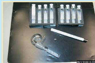
Overview of the measurement cuvettes used. Eight measurement cuvettes, filled with liquid medium and fixated bacteria at increasing concentrations for calibration purposes. One measurement cuvette with air reservoir for the growth measurement
