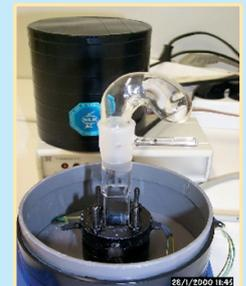
Optical sensor head breadboard with cuvette in measurement position
