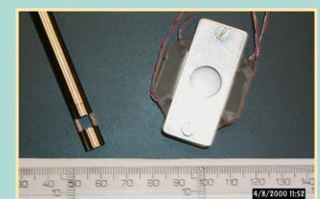
Examples of future application. Submerged probe and glass sensor integrated with bioreactor
