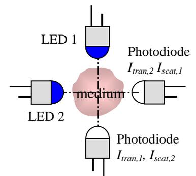
Figure-1. Dual ratio turbidity sensor concept
