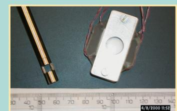
Examples of future application. Submerged probe and glass sensor integrated with bioreactor
