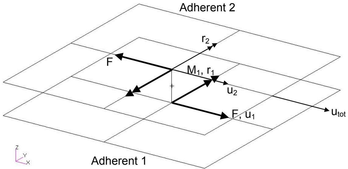
Figure 8. Parameters of analytical model for single bolt, single lap joint.
