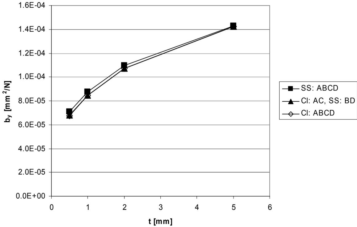
Figure 3. Parameter  $b_y$  as function of adherent thickness  $t$  for various boundary conditions for fine mesh.
