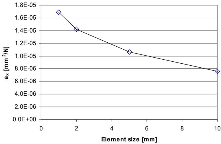
Figure 4. Parameter  $a_x$  as function of element size.
