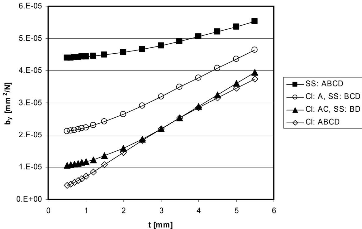
Figure 2. Parameter  $b_y$  as function of adherent thickness  $t$  for various boundary conditions for coarse mesh.
