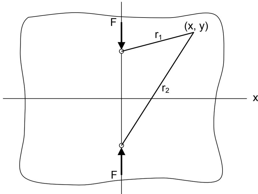
Figure 7. Parameters for a plate loaded by a point load.
