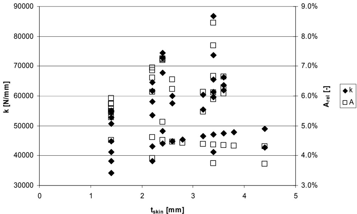
Figure 10. Bolt spring constant k and relative area of beam as function of the skin thickness for various doubler thicknesses.
