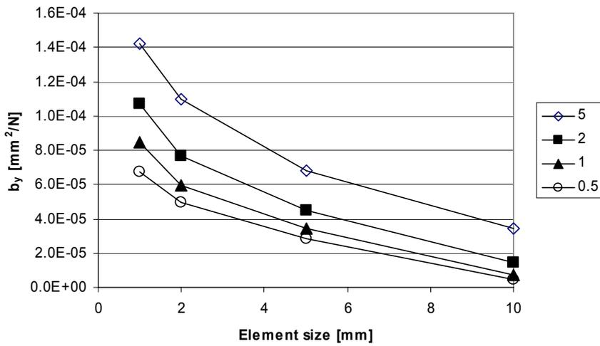
Figure 5. Parameter  $b_y$  as function of element size for various adherent thicknesses for all clamped boundary condition.
