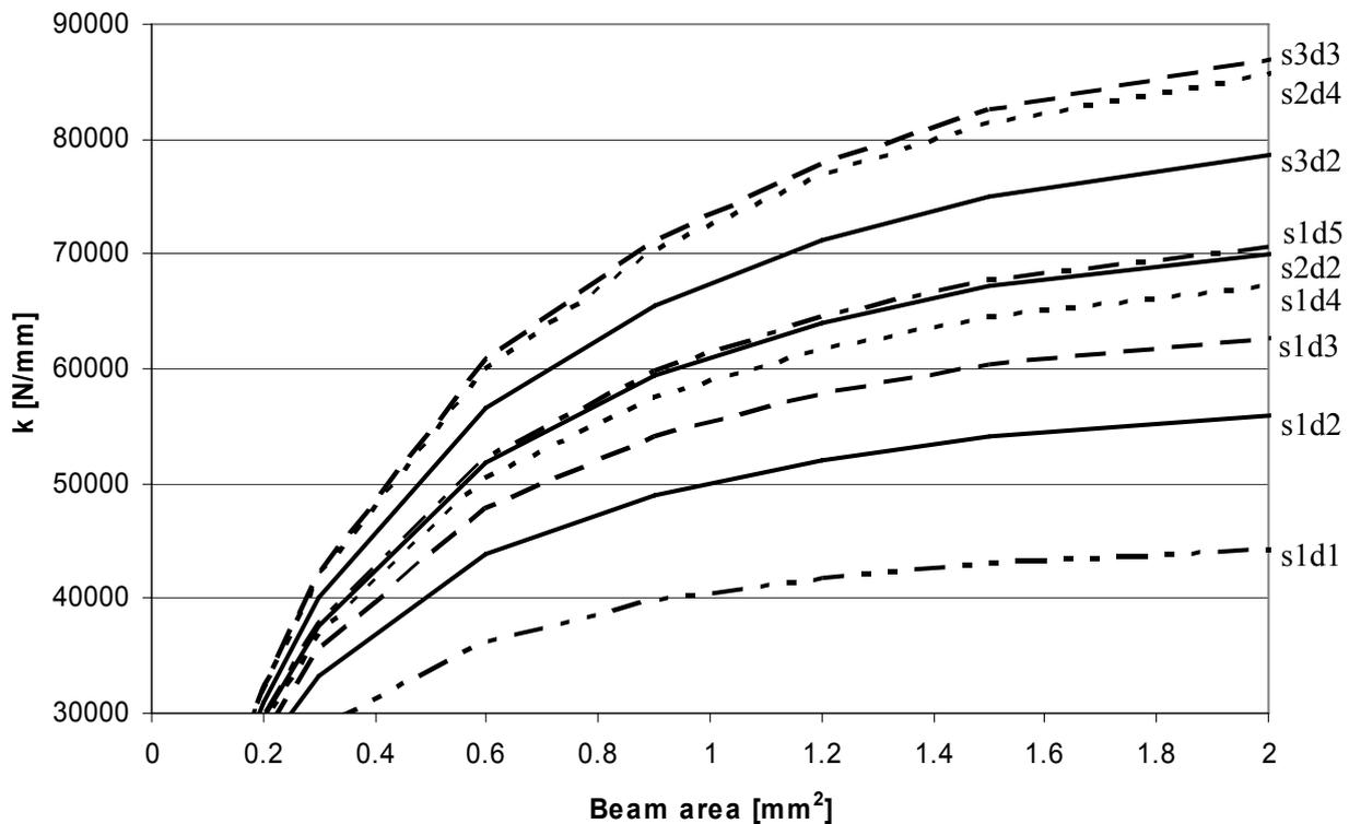
Figure 9. Bolt spring constant  $k$  as function of the beam area for various combinations of skin and doubler thickness.
