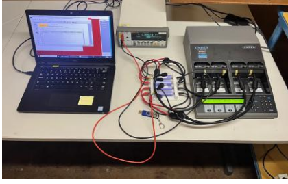
Figure 7: The experimental setup used to test the battery cells
