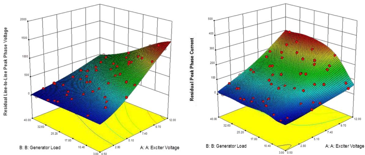
**Figure 10. Design space residual maps for generic generator model and experimental results; line-to-line peak phase voltage and peak phase current.**
