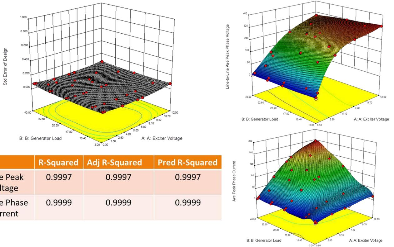
Figure 9. Experimental statistical model standard error and resulting voltage and current response surfaces derived from experimental test plan.
