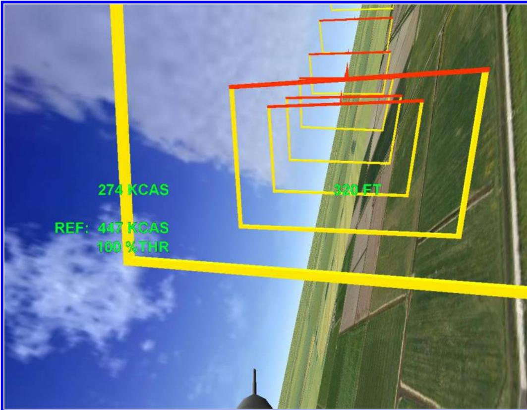
**Figure 16 Tunnel in the sky and HUD showing a tight turn. The red side of the tunnel markers indicates ‘up’ direction in the aircraft body frame. On the bottom left of the HUD, the airspeed and throttle position used during the original flight are shown for reference.**
