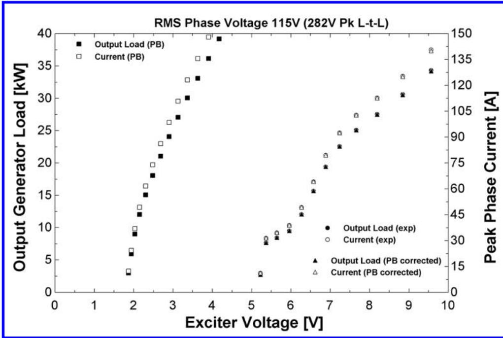
Figure 11. Residual map correction for generic generator physics-based model to experiment at a controlled voltage of 115V (282V line-to-line peak phase voltage).
