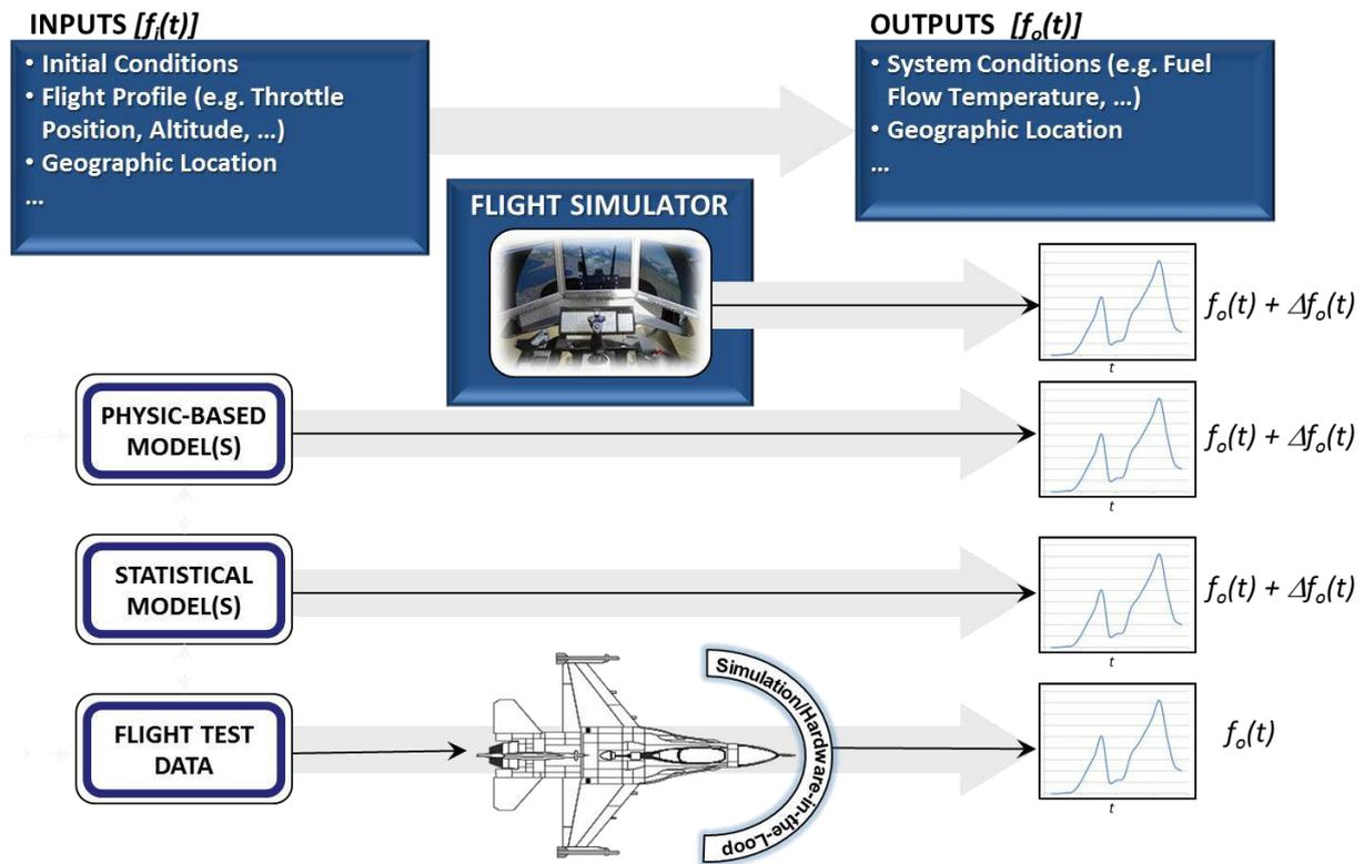
Figure 19. IEPM Laboratory validation testing approach.
