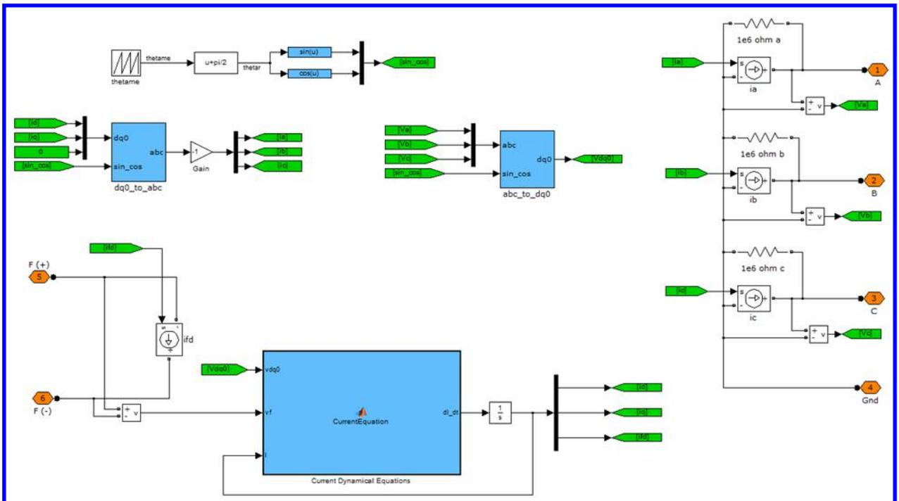
Figure 5. 2-stack synchronous generator model (synchronous generator and exciter blocks).
