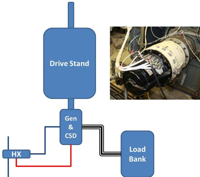
Figure 8. Experimental testing configuration showing installed generator and constant speed drive (CSD).
