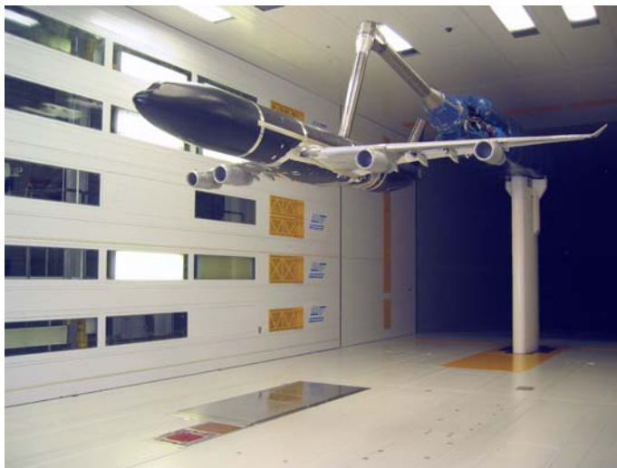
Figure 2: Test set-up in DNW closed test section, with wall arrays on the tunnel floor.
